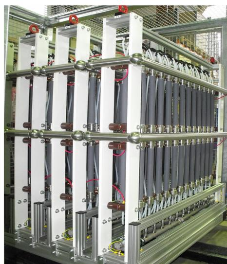
Three Resistor Modules in HV Housing
