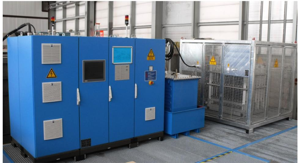
Klystron Replacement Dummy at Modulator Commissioning Site
